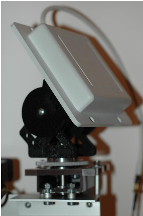
Figure 4: ServoCity mount with 8dBi 2.4GHz antenna installed
